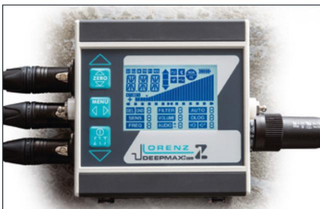
From time to time **ZERO** has to be pushed shortly to recall the audio threshold setting during operation.
